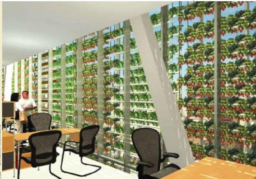
A vertically integrated greenhouse, conceived by New York Sun Works, Kiss + Cathcart, and Arup Engineers, would consist of hydroponic troughs that would move up and down within the airspace of a double-skin facade. In addition to growing vegetables for sale, the system would contribute to the thermal and acoustical insulation of the building.
